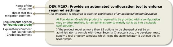
Figure 2: Components of a typical mitigation
